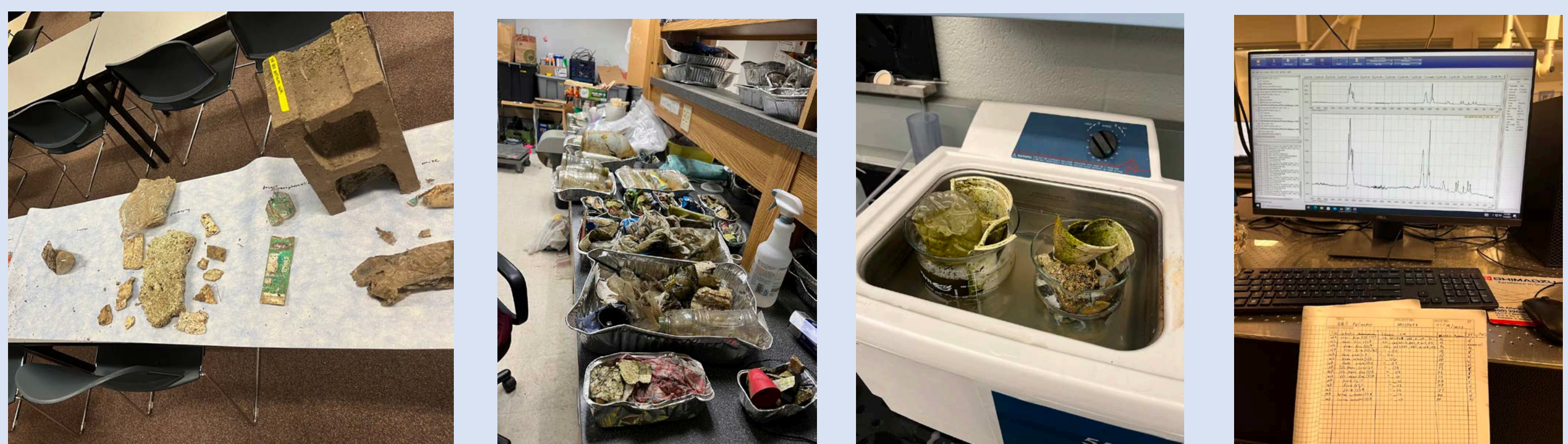
Figure 2. We count and categorize, dry, and sonicate on the water-perimeter and transect plastics in order to prepare for IR.
